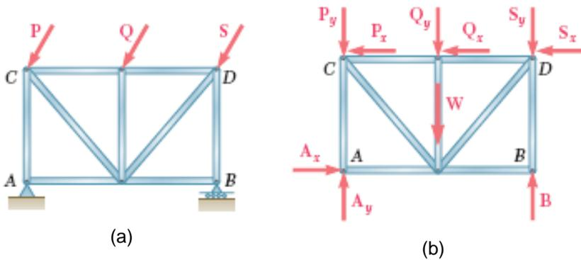
$$\begin{aligned} \Sigma F_x &= 0 \\ \Sigma F_y &= 0 \\ \Sigma M_A &= 0 \end{aligned}$$
